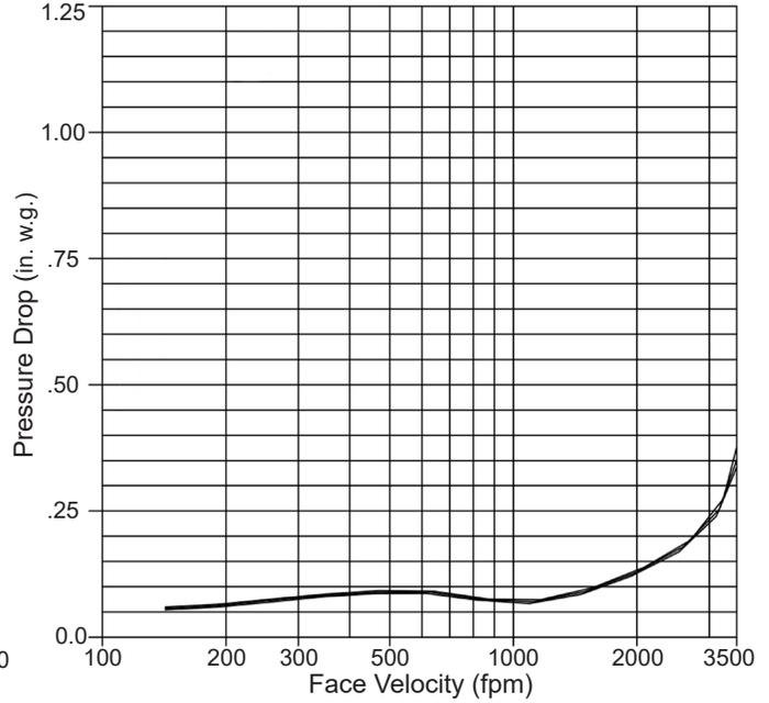
Typical performance for Model PRI9 backdraft damper size tested 42"W x 42"H furnished with counterweight to assist opening.
